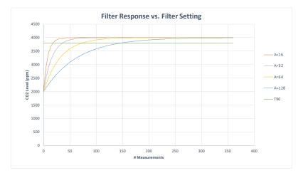
The graph above shows the effect of the filter on response times. Increasing the filter setting increases the measurement output response time.  $T_{90}$  is the time to 90% of reading. The CozIR®-LP2 takes 2 readings per second. The CozIR®-LP2 sensor will also output the raw unfiltered  $CO_2$  measurement data. This data can be post processed using alternative filter algorithms.
